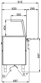
D = Drain El = Electrical inlet (power)
